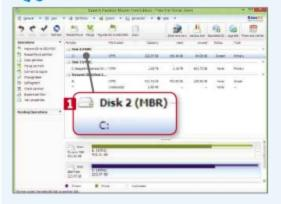
If Windows is already installed on your hard drive and you haven't previously partitioned it, you will need to resize the Windows partition to make room for the new operating system. EaseUS Partition Master Free (www.partition-tool.com) is a good tool for the task. Click 'Go to home page' and select your system drive. [1]
